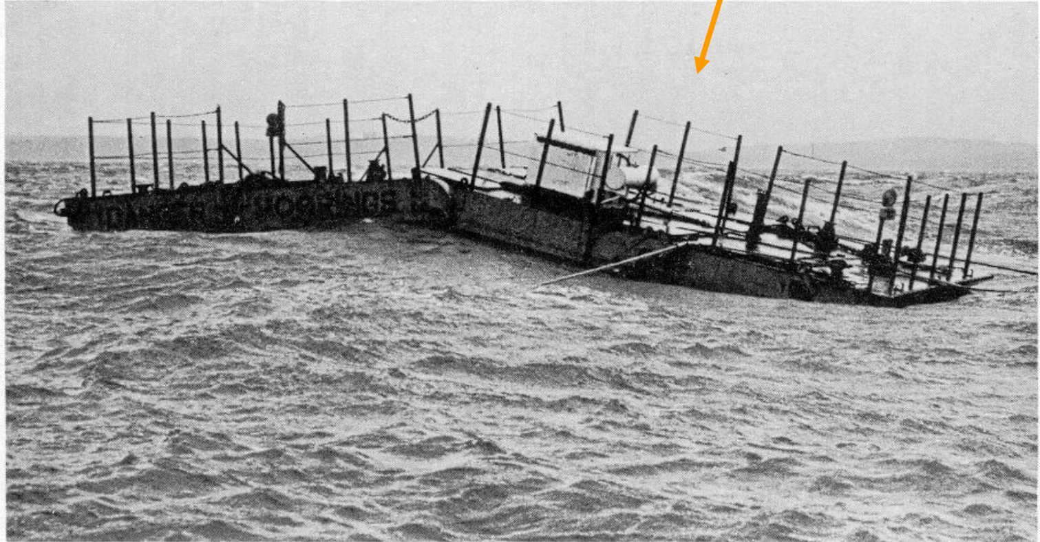
Figure 7.2 The ship with a broken back. Cockerell's 1/10th scale raft working in the Solent.
